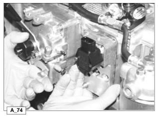
Operate the stop control lever repeatedly to make sure the system is running smoothly.
