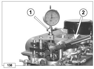
Assemble tool serial no. 1460 - 266 made up of lever **2** serial no. 1460 - 275, of a dial indicator **1** serial no. 1460 - 274 inserted in a dial indicator holder serial no. 1460 - 270.
