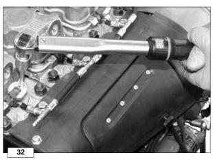
O The fixing bracket screws must be tightened to 10 Nm using a torque wrench.
