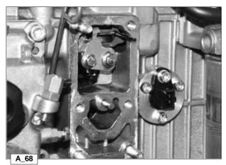
Remove the cover supporting the sensor and the fuel pump.
