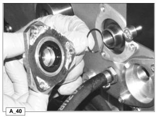
Refit the oil feed bushing to the variator, placing the oil seal support ring in between. Replace the seal.
