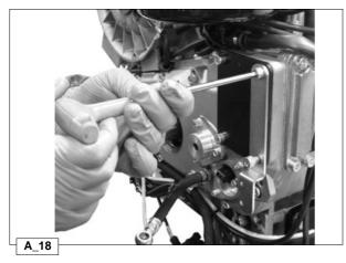
Loosen the two screws M8 to disassemble the solenoid valve support bracket.
