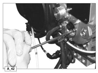
O Attach the sensor using screw M6 to a torque of 8 Nm.
