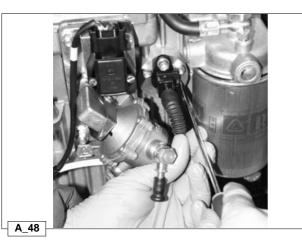
To assemble the phase sensor connector press the locking spring.
