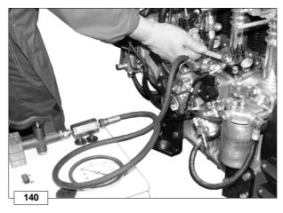
To the injection pump connect the high-pressure pump serial no. 1460 - 273 supplied by a tank whose fuel level is at least 100 mm above the injection pump.
