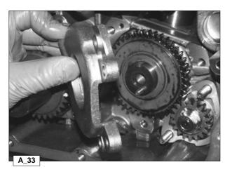
Remove the shoulder housing of the idle gear that drives the speed governor.
