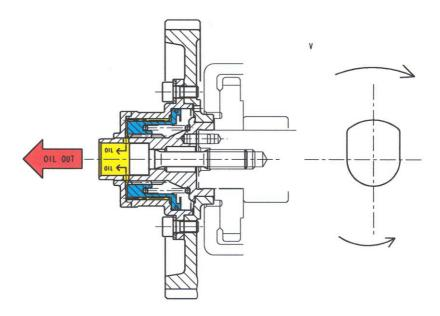
Our system is able to actuate any intermediate advance, regulating the oil pressure. When the set level is reached, the oil exerts the right force to compress the spring at the right height to move the plunger appropriately, thus achieving the required rotation (angular advance).
