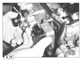
Look through the upper inspection hole on the cover to make sure that the pin 1 is correctly inserted into the fork 2.
