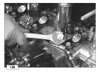
Unscrew the fuel supply union for the injection pump of the cylinder which is to be worked on.
