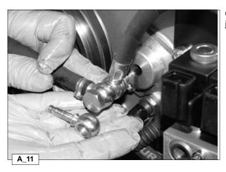
On the opposite end of the block of pipe 19 is the variator lubrication jet attached to the pipe by a click clamp.
