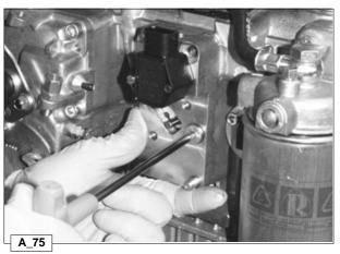
Replace the screws and nuts in the cover in the opposite order to when they were removed and
