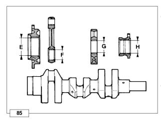
Main bearing and connecting rod big end bearing inside diameter
