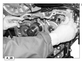
Remove the timing cover seal.
