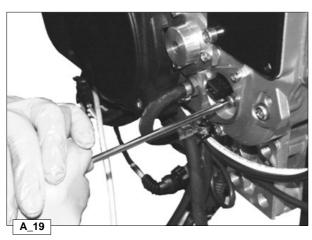
Loosen screw M6 to remove the speed sensor from its support.
