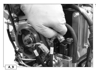
To remove connectors, press the stop tabs and draw upwards.
