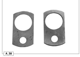
Example of where to insert the air gap adjustment shims.
