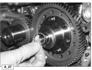
Pay attention to the oil seal support ring when disassembling the timing cover.
