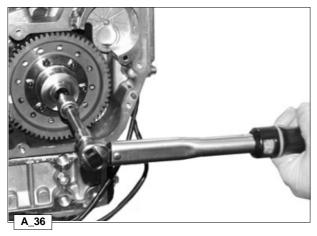
Assemble the variator onto the end of the camshaft taking care to properly insert the timing pin into place and ensuring that the variator comes into contact with the surface of the speed governor idle gear.
