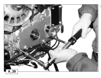
O Tighten the screws to a 25 Nm torque.
