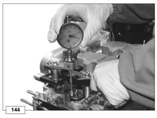
Press the lever to bring the valve into contact with the piston crown. By joggling back and forth clockwise and anticlockwise, find the dead centre via the dial indicator and then reset to zero.
