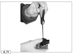
Tighten only one screw on the position sensor to keep it in the right position.
