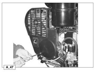
O Replace the built guard and tighten to 15 Nm.
