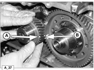
Assemble the timing control gear onto the crankshaft so that reference mark  ${\bf A}$  is lined up with the two reference marks  ${\bf B}$  on the idle gear installed on the camshaft.
