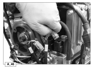
Insert the solenoid valve connectors following the references ( ${\mbox{IN}}$  and **OUT**) shown on the cables and on the solenoid valve block.
