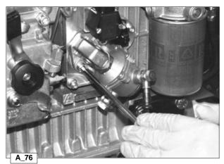
Refit the fuel pump after replacing the seal; tighten the screws to 25 Nm.
