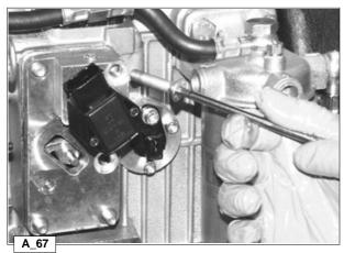
Unscrew the last screw (flathead) after rotating the sensor anticlockwise.
