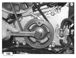
Rotate the crankshaft clockwise on the timing belt side and position the relevant cylinder piston at top dead centre.
