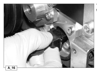
To remove the speed sensor cable connector press the spring as shown in figures **A\_16** and **A\_17** and draw upwards.
