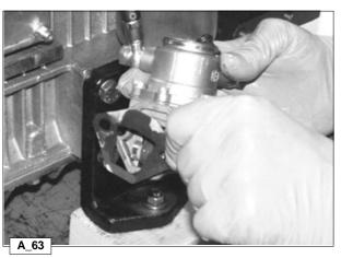
When reassembling, replace the sealing gasket.
