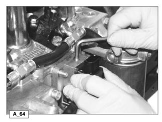
Remove the conical inspection plug.
