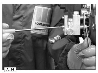
To remove the solenoid valve block from the support bracket, unscrew the two screws M 5.
