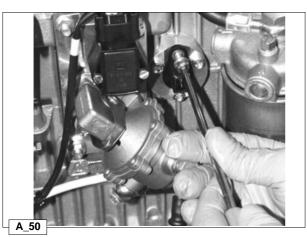
O Loosen screw M6. When refitting, tighten to 8 Nm.
