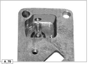
Insert the fork into the slot in the support. Rotate the sensor body 180°, keeping the fork in the position shown in figure A  $\_70$ .
