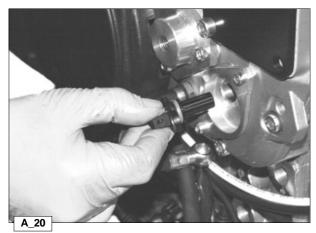
Draw he speed sensor outwards, being careful not to damage the rubber seal ring.
