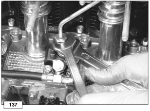
Use a 19 mm box wrench to lock the injection pump union and a 17 mm box wrench to loosen the union of the injector pump high-pressure pipe.
