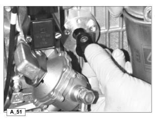
Remove the sensor from the support taking care not to damage the O-ring.
