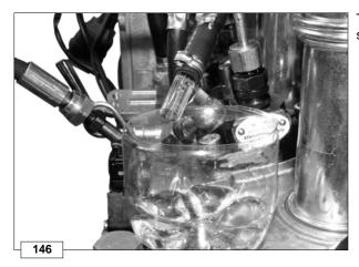
The capillary tube shows when the fuel is flowing out, thanks to its small transparent slot.
