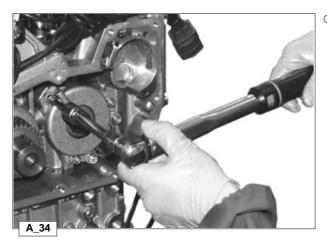
O After refitting the housing tighten the screws to 20 Nm using a torque wrench.
