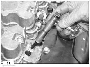
These operations are necessary when checking injector calibration or when replacing it.
