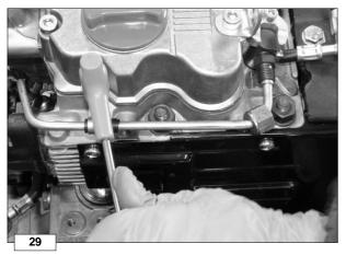
Unscrew the screw fastening the clamp of the high-pressure pipe using a 4 mm hexagon screwdriver.
