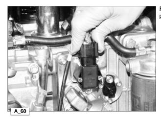
Remove the connector from the position sensor on the injection pump control rod.
