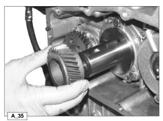
Remove the distribution control gear from the crankshaft.
