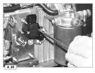
Unscrew the two screws to disassemble the injection pump rod position sensor.
