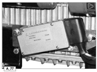
Correct assembly position of the control unit that runs the engine variator.
