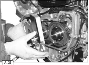
After loosening the screws, remove the timing cover.
