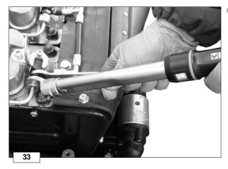
O The high-pressure pipe union must be tightened to the injector union to  $20 \div 25$  Nm using a torque wrench.
