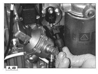
Remove the connector from the sensor.
