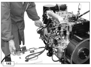
Rotate the crankshaft anticlockwise until diesel starts to flow out from the capillary when the high-pressure lever is pressed.
