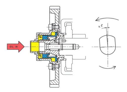
Fig. A\_3. Injection timing device: moving from actuation of an advance to resting position.
