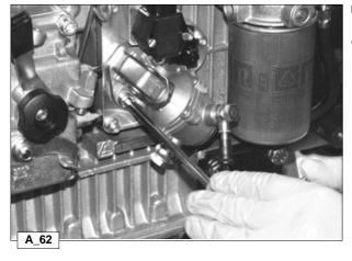
Unscrew the two screws to disassemble the fuel pump;
