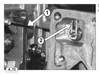
Set the cover against the crankcase so that the injection pump rod drive pin 1 is inserted between the two prongs of the fork 2.
