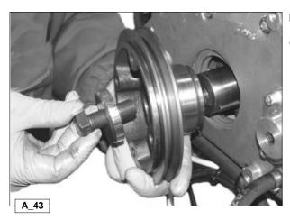
Reassemble the blower control pulley onto the crankshaft.
