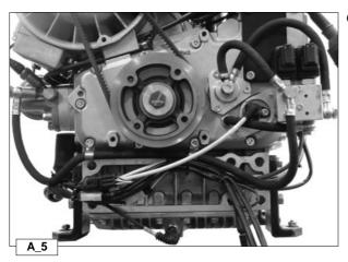
Overall view of variator speed sensor and hydraulic circuit.
