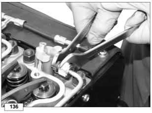
Use a 14 mm box wrench to lock the injector union and a 17 mm box wrench to loosen the union of the injector pump high-pressure pipe.
