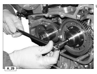
Unscrew screws M10 on the variator to the camshaft.
