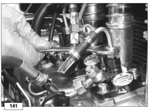
Insert the capillary tester serial no. 1460 - 024 onto the injection pump union where the high-pressure pipe is usually connected from the pump to the injector.
