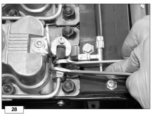
To release the injector union from the high-pressure pipe, use two box wrenches (14 and 17 mm).
