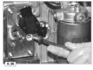
Remove the three flanged nuts and the flathead screw.
