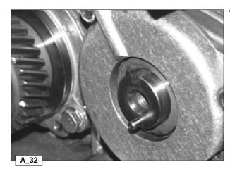
View of the camshaft ends with pin inserted.
