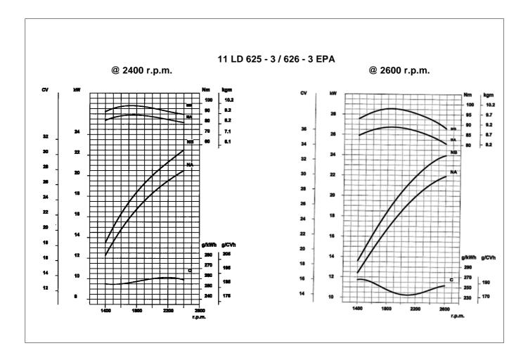
N (80/1269/EEC - ISO 1585) - AUTOMOTIVE RATING: Intermittent operation with variable speed and variable load.
