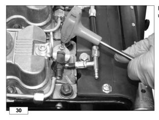
Remove the forked bracket fixing the injector to the cylinder head using a 5 mm hexagon screwdriver (see photo 29 - 30).
