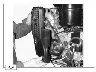
After loosening the screws, remove the alternator belt guard.
