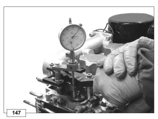
After finding the delivery start point (when fuel stops flowing from the capillary), press the lever and use the dial indicator to check how many millimetres the piston has moved from the top dead centre. Check static injection advance using the conversion table from millimetres to degrees.
