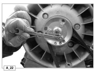
Blower belt alternator - Disassembly
