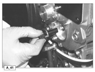
Replace the speed sensor taking care not to damage the O-ring.
