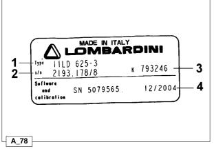
Example of adhesive plate on the control panel
