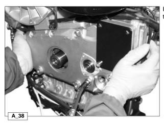
Replace the timing cover, placing a new seal and lining up with the two centring pins.
