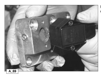
Rotate the position sensor shaft to direct the fork on the side opposite the connector.
