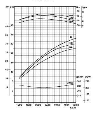
N - 80/1269/CEE- ISO 1585, Gross automotive rating- intermittent operation with variable speed and variable load.
