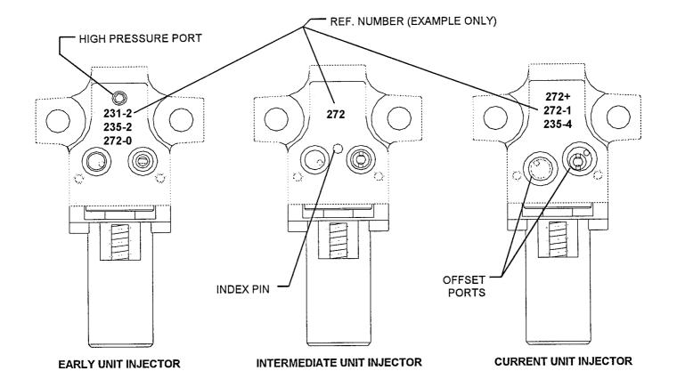
LOMBARDINI CONTINUALLY DEVELOPS THE FOCS DIESEL LINE. CONSTANT RESEARCH AND DEVELOPMENT IS CARRIED OUT TO IMPROVE OVERALL PERFORMANCE OF FOCS PRODUCTS. AS SUCH, THE DESIGN OF THE FOCS UNIT INJECTOR HAS CHANGED DURING THE DEVELOPMENT PROCESS. THE FIGURE ABOVE PROVIDES A REFERENCE FOR THE THREE(3) DIFFERENT VERSIONS OF THE FOCS UNIT INJECTOR TO DATE.
