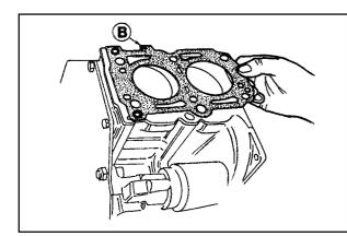
Match the piston protrusion dimension determined above with dimension(A) from the chart. Install the corresponding head gasket. If a head gasket cannot be chosen based upon the piston protrusion measured, check the connecting rod length, rod bearings, wrist pin bushing, etc. for the cause of the problem.
