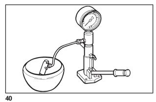
check the time it takes to drop. The pressure must drop to 150 to 100 Kg/cm<sup>2</sup> withinn 6 to 40 seconds.
