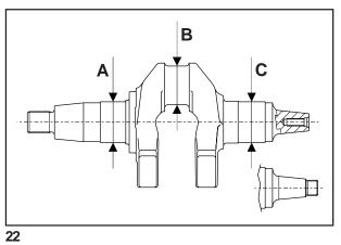
Undersized bearings can be mounted without any reaming work required.
