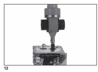
Grinding-in must always be carried out when new valves or housings are mounted. Valve housings oversized on the outside by 0.5 mm are available.
