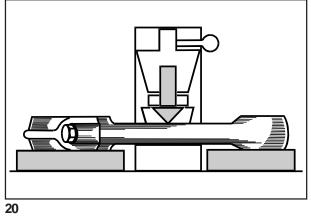
The operation is carried out by applying a calibrated pressure to the convex side in the middle of the connecting rod stem set on surface plates (fig. 20).
