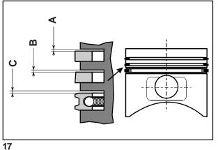
Piston ringMax. wear mm1st CompressionA = 0,222nd CompressionB = 0,193rd Oil scrapperC = 0,16
